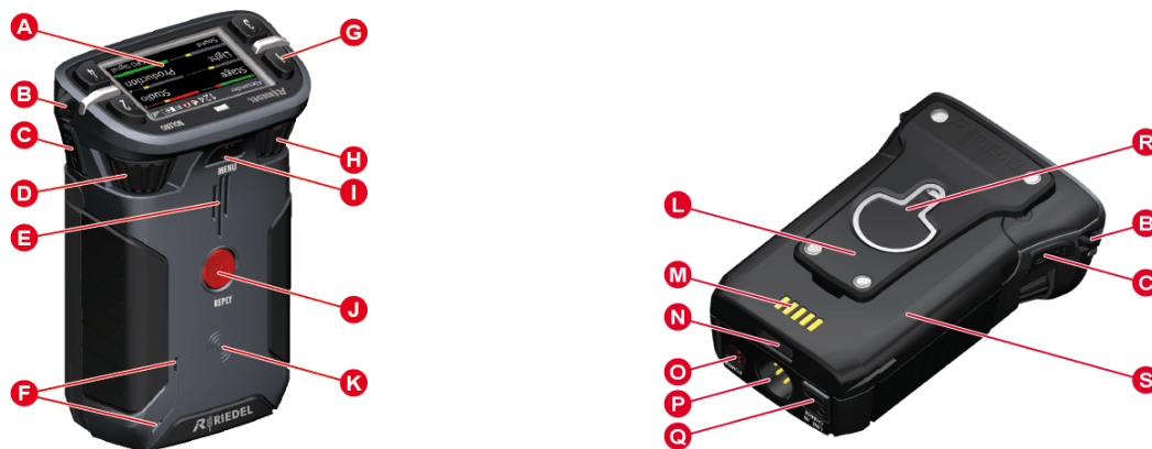
Figure 160: Beltpack – Operating Elements (front/top, rear/bottom)
