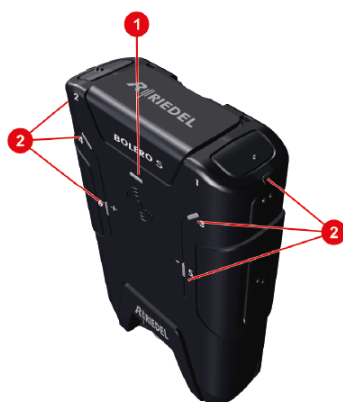
Figure 208: S-Beltpack – Status LEDs (top)
