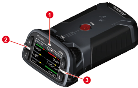
Figure 164: Beltpack – Status LEDs (top)
