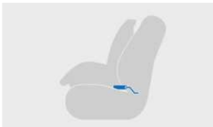
Child restraint installed using ISOFIX [1]
