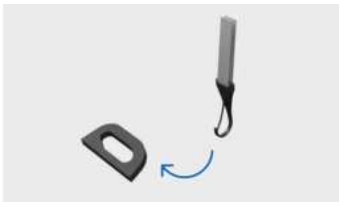
Fastening tether to lower tether attachment point
