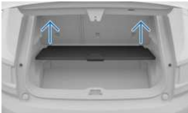
Illustrated guide to removing the cargo hatch.
