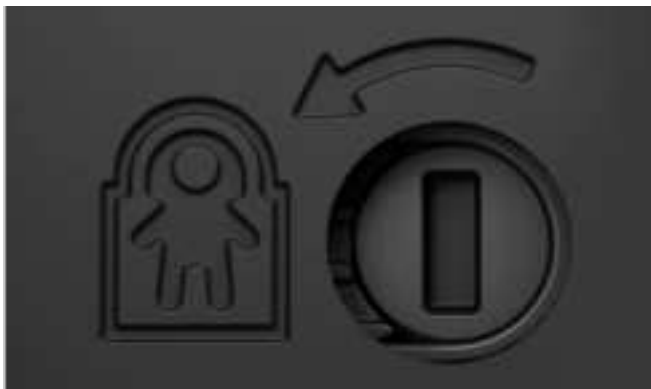
Child lock with turning direction for activation.
