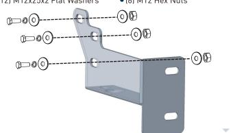
(Driver Side) Secure the bumper. Repeat this step for the opposite of the bumper. Tighten all hardware.
