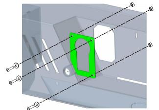
(Driver Side) Install the mounting brackets. Repeat this step for the opposite of the vehicle. Do not fully tighten hardware to allow adjustability.
