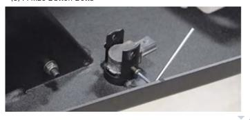
Step 3 Install the trailer plug bracket to the bumper. Choose the correct bracket for the 7 way trailer plug. Attach bracket to 7- way connector.
