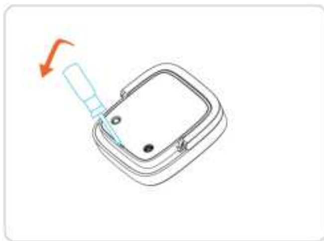
② Pry open the bottom cover.
