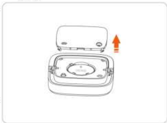
③ Remove the bottom cover
