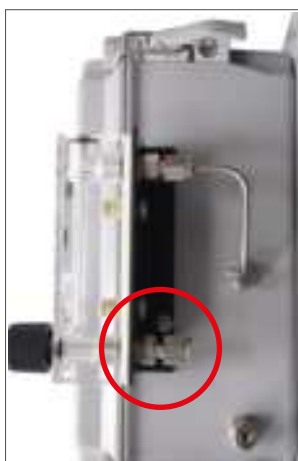
Figure 4 - Gas inlet (analyzer's right side elevation)
