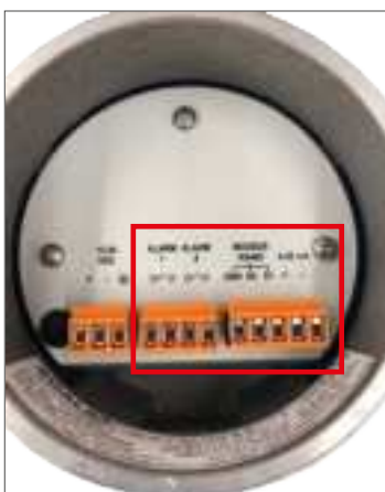
Figure 3 - Wiring your analyzer
