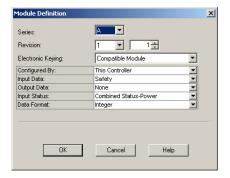
Setting the output data to None means that you cannot use the Test Outputs as standard outputs, which is appropriate in this example. This configuration saves one controller connection, because we are using only the input connection.
