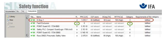
The Fault Exclusion (green) had no effect on the calculations. The CAT. 3, PL d, and DCavg 60% were manually entered to reflect the effect of the E-stops wired in series.
