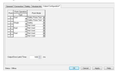
6. Click Output Configuration and configure the module as shown.
