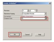
Chassis size is the number of modules that are inserted in the chassis. The 1734-AENT adapter is considered to be in slot 0, so for one input and one output module, the chassis size is 3.
