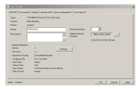
13. When the Module Definition dialog box opens, change the Output Data to None verify that the Input Status is Combined Status-Power, and click OK.
