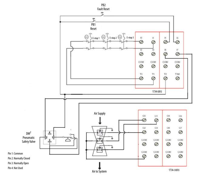
Pins 1 and 3 are connected when air pressure is present and the valve is Ready to Run.
