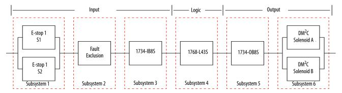
The SISTEMA calculations confirm that the proposed safety functions are capable of achieving the required level of protection CAT. 3, PLd.
