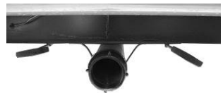
Black/Grey Tank Drain & Valves
