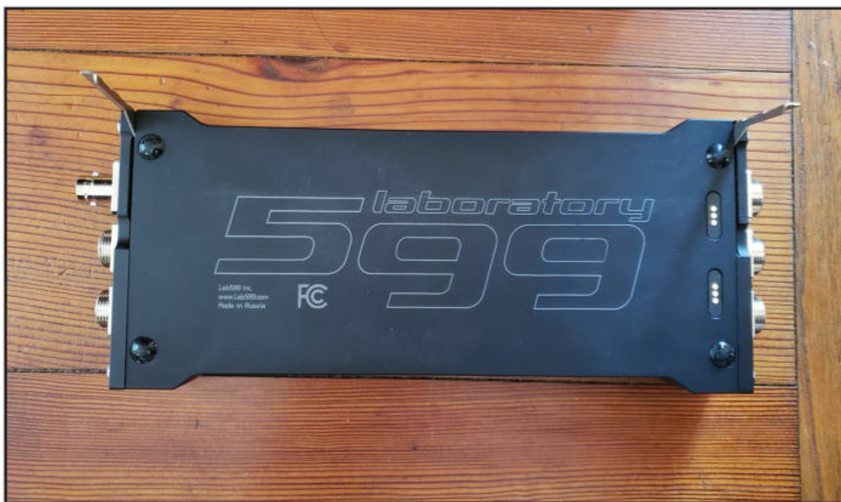
Photo D. Backside of the TX-500 with its metal kickstands deployed. The two tabs on the right side are connections for the detachable battery pack (available soon).
