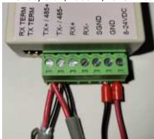
2-Wire Daisy-Chain, No SGND, No Termination
