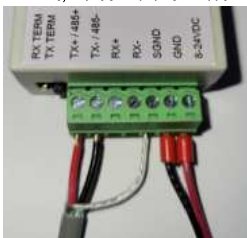
2-Wire, with SGND and Termination
