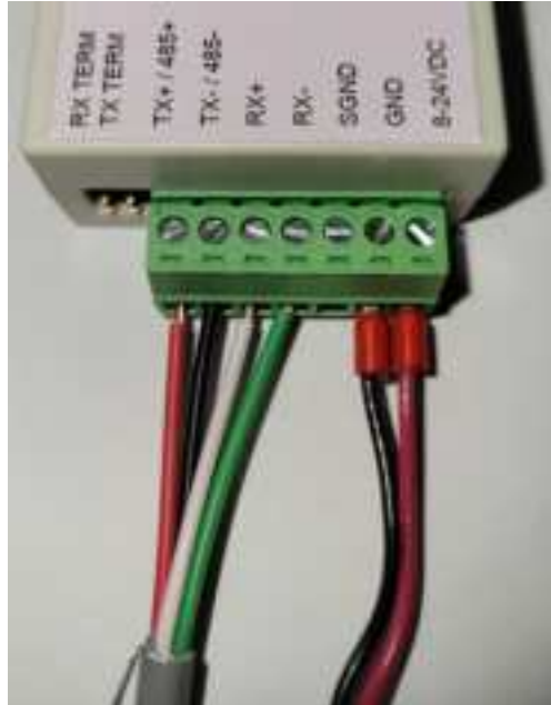
4-Wire, No SGND, No Termination
