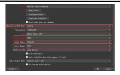
Notes: If there is no video format YUY2 after setting above, check the USB 3.0 port connection. Make sure it is linked to USB 3.0 port on PC by a USB 3.0 cable. (USB 3.0 cable or port is standard in blue while USB 2.0 is in black). If the captured picture flashes, change the video format to YUY2.
