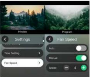
Turn on "Auto", and the device will automatically adjust the fan speed. Turn off "Auto", then you can manually adjust the fan speed, which supports four adjustable speeds.
