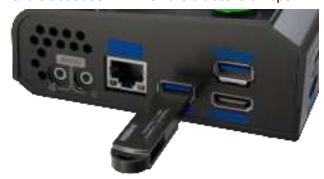
Insert the USB flash disk into the USB recording port of the mini-ISO with the RECORD silkscreen. Format your hard disk or USB flash drive before using the recording function. To format the hard disk on the mini-ISO, proceed as follows:
