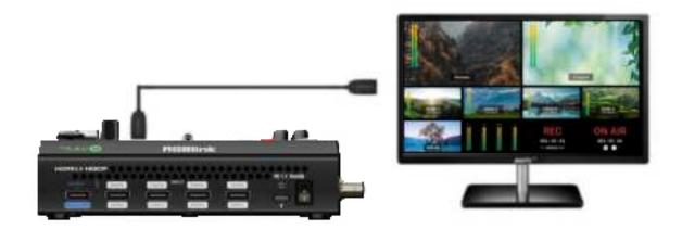
HDMI multi-screen output not only supports multi-picture monitoring, but also supports the choice of fixed output of a particular input signal or directly selecting the main output of the signal. You can make adjustments through the output settings in the menu for PRE and PGM switching and switching between the various input signals.
