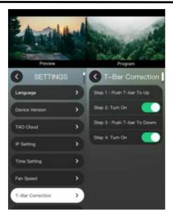
The user can complete the calibration by following the four steps.
