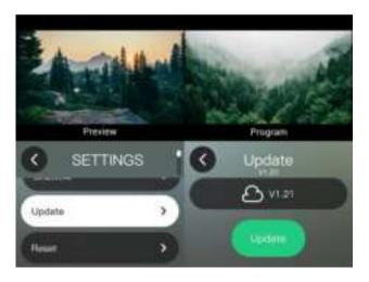
In this interface, you can press the "Update" on the right side to upgrade the mini-ISO (See <u>6.3 Upgrade Guidelines</u> for details on the steps to upgrade the device). Please make sure your network is working during the update.
