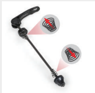
Take out the quick-release clamp, pls pay attention to the direction of spring.
