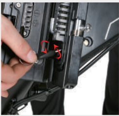
Turn the key to lock or release the battery lock
