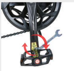
Tighten the right pedal "R" clockwise
