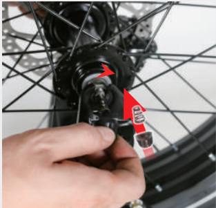
Tighten the quick disassembly in the direction
