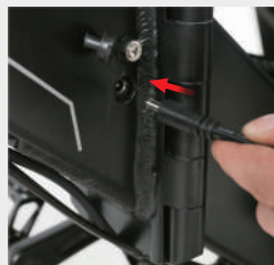
Method 1: Charge the electric bike directly in the direction indicated by the arrow
