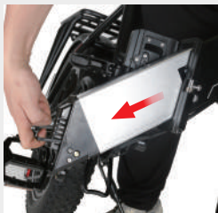
Remove the battery in the direction
