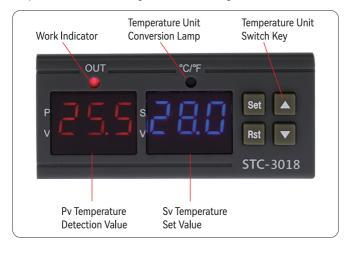
**6.Temperature Adjustment Mode:** Press the "SET" button once, and the SV setting value starts to flash. Press the "Up" or "DOWN" button. After the specified temperature is set, press the "SET" button to save.
