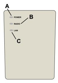
A: Power LED = Green indicates the presence of line power or power over Ethernet
