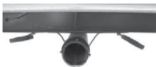
Black/Grey Tank Drain and Valves
