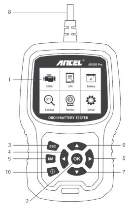
1) LCD DISPLAY - Displays test results. 2.4" TFT 262K true color, 320\*240
