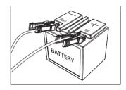
2) For a proper connection, rock the clamps back and forth. The tester requires that both sides of each clamp be firmly connected before testing.
