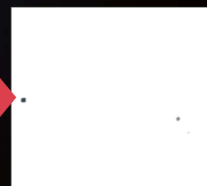
Removes the striped pattern and reveals only the foreign particle
