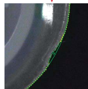
The tool reliably detects even the most subtle nicks along the profile, a defect otherwise considered difficult to detect.
