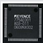
Low angle lighting enhances the printing and leads.
