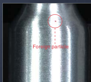
Foreign particle detection on a rounded metal surface
