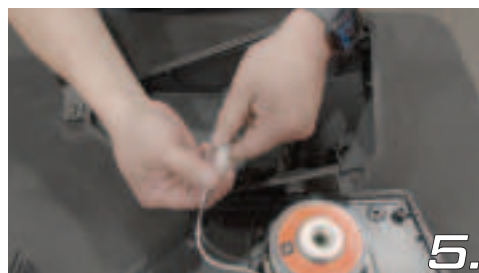
Unplug the OEM speaker from the enclosure
