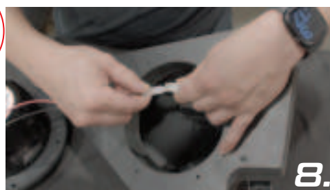
Plug in the speaker to the OEM plug
