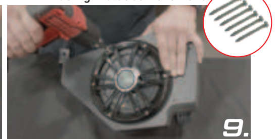
Place the speaker into the enclosure and secure using included hardware
