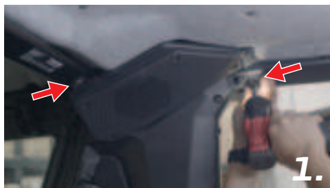
Remove the two screws shown here
