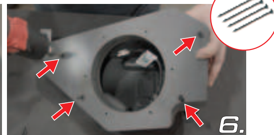
Place the UTV Stereo speaker mount onto the OEM enclosure and secure using included hardware
