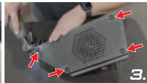
Remove the 4 screws on the speaker grille
