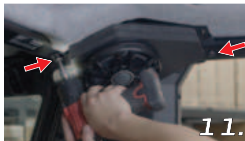
Use the same OEM screws to secure the enclosure to the roof
