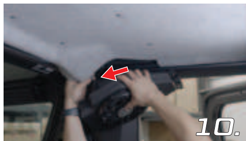
Place enclosure back into the vehicle and plug in before securing to the roof
