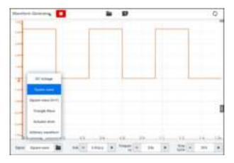
Figure 9-91 Signal Mode Setting Screen
