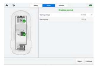
Figure 12-8 Starter Test Result Screen
