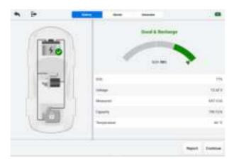
Figure 12-7 Battery Test Results Screen
