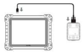
Figure 16-1 Connecting MaxiSys Tablet and Hand-held Inclinometer
