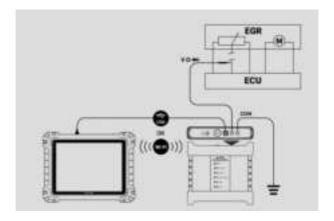
Figure 9-92 DC Voltage Connection Diagram
