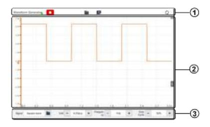
Figure 9-85 Waveform Generator Menu Screen
