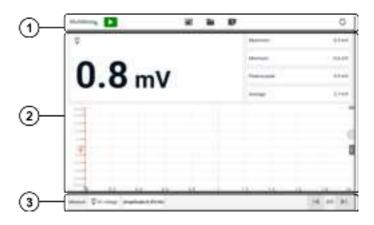
Figure 9-63 Multimeter Menu Screen
