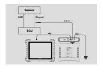
Figure 9-97 Arbitrary Waveform Connection Diagram
