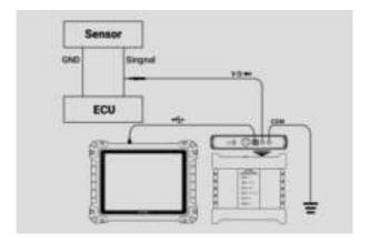
Figure 9-96 Triangle Waveform Connection Diagram
