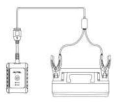
Figure 12-4 Battery Tester Connection Example 2
