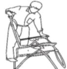
3. To recline, push back with your body while elevating your feet. Resistance tabs on the arms allow the chair to stop in any position.
