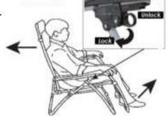
To return to the upright position, pull forward with your body while pushing downward
