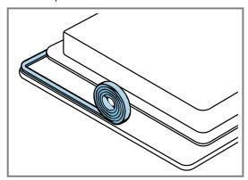
Move the shorter part of the adhesive seal strip supplied into the area underneath the front part of the hob. If necessary, cut the adhesive seal to the required length.
