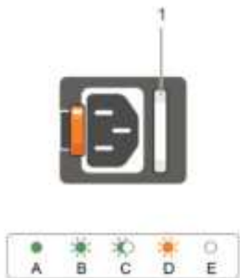
Figure 17: Power Supply unit Indicators
