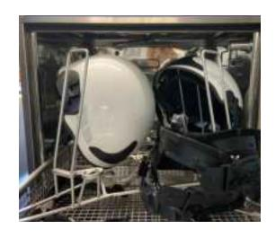
Processing helmets in a dishwasher is uncomplicated in terms of handling. As there is no movement mechanism, no specific protective measures need to be taken. The helmets are placed in the appliance completely equipped (except for electronic components) and cleaned in the same way. Depending on the design of the baskets, several helmets can be loaded next to each other at the same time.
