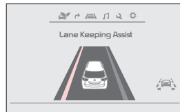
When the LKA sensor detects the vehicle moving outside of the lane being traveled in, a yellow indicator will illuminate either on the left or right lane (shown in both images above)
