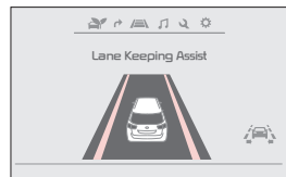
When the LKA sensor detects the lane traveled in, both lanes are illuminated
