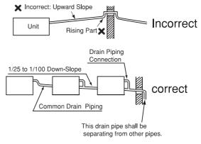
Fig. 6.1 Drain Piping
