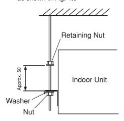
Fig. 4.5 Sling Bolts and Nut
