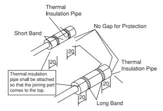
Fig. 5.3 Insulating Pipes
