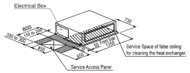
Fig. 4.1 Operation and Installation Space
