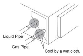
Fig. 5.2 Blazing Pipes
