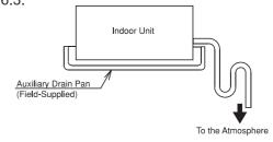
Fig. 6.3 Auxiliary Drain Pan
