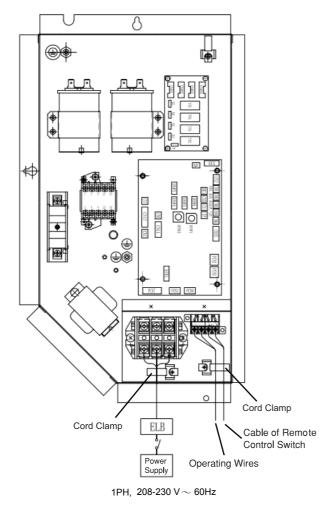
Fig. 7.2 Electrical Wiring Connection
