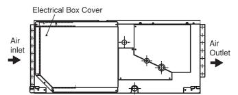
Remove the fixing screws for electrical box cover.
