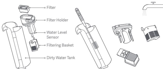
4. Reinstall the filter and the filtering basket onto the filter holder, and put the filter holder into the dirty water tank. Then install the dirty water tank into the vacuum. The tank is secured in place when you hear a click.
