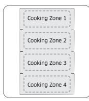
The Flex zone is the large cooking area located on the left side of the hob (see the figure below) that is specially designed to accommodate multiple pots and pans of varying shapes and sizes at once. The Flex zone has four zones that are operated by individual inductors, allowing you to cook regardless of where cookware is placed on a cooking zone.
