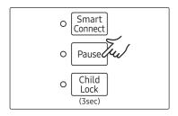
2. Touch the **Pause** key for 3 seconds within 10 seconds of pressing the **POWER** key.
