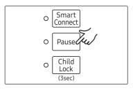
The **Pause** function simultaneously switches all cooking zones that are switched on to the low power setting. This function can be used to briefly interrupt and then continue the cooking process e.g. to take a telephone call.
