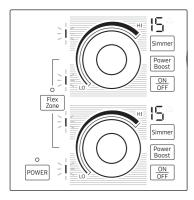
The Flex Zone indicator uses pan detection to display the active zone when the Flex Zone function is enabled
