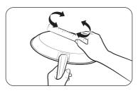
The cookware used with the cooktop surface should have flat bottoms that make good contact with the entire surface of the Cooking Zone. Check for flatness by rotating a ruler across the bottom of the cookware. Be sure to follow all the recommendations for using cookware.
