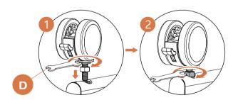
Turn the hex bolts with wrench, and screw the casters into the base, finally fix the nuts with wrench.
