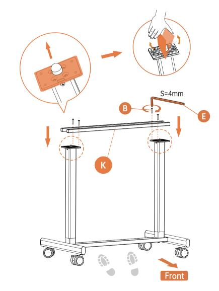
Note:Remove the plastic cap before installing to the cross bar .
