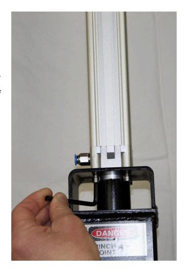
Finished product should look like this. Connect the two air tubes and the assembly is complete.
