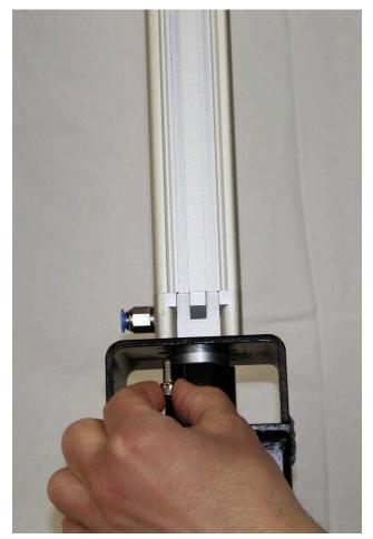
With a lock washer on each screw, hand-thread all four of into the air cylinder.
