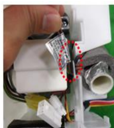
4. Remove the wire from the auger motor. - Remove drain line.
