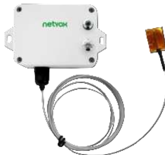
R718BP - Patch probe -50° to 150°C
