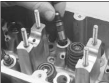
8.20c . . . then lift out the hydraulic tappets
