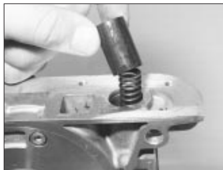
14.27b . . . and remove the sleeve . . .
