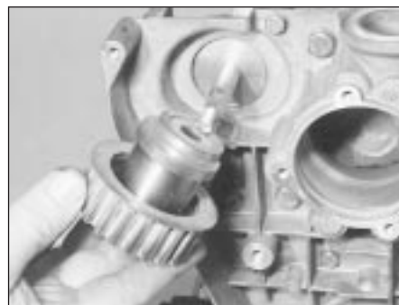
14.8 Removing the timing belt tensioner (M40 engine)
