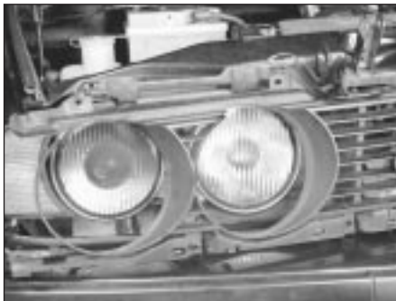
9.14 Remove the screws and pull the side grille assembly straight out
