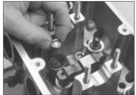
8.20b . . . and thrust discs . . .
