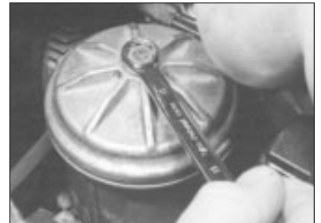
6.17a Unscrew the bolt . . .
