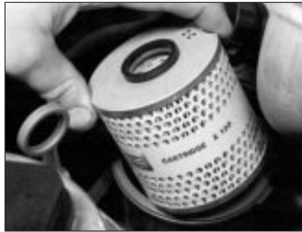
6.17c ... and lift out the cartridge
