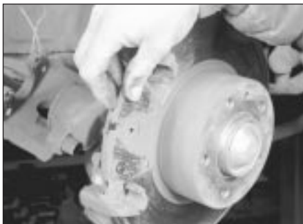
3.5m Remove the outer brake pad - to fit the new pads, reverse the removal procedure
