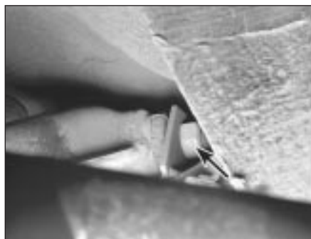
13.6 Nut (arrowed) for the outer pivot bolt
