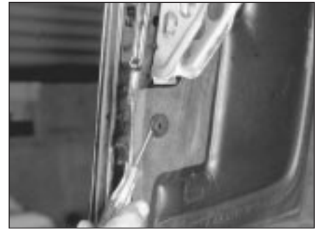
10.8b . . . prise the retainer out
