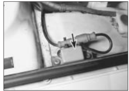
18.3 The SRS system crash sensors (arrowed) are located in the engine compartment - check the wiring regularly for damage
