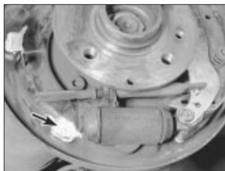
6.11 Before you fit the new shoes, apply some high-temperature brake grease to the friction surfaces where the inner edge of the shoe slides on the brake backing plate - when you refit the automatic adjuster mechanism, make sure each end engages properly with its respective notch in the brake shoe
