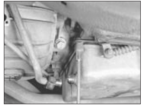
28.6 Use a socket and extension to remove the bolts and brackets
