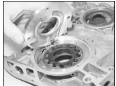
14.21b . . . and remove the oil pump cover (M40 engine)
