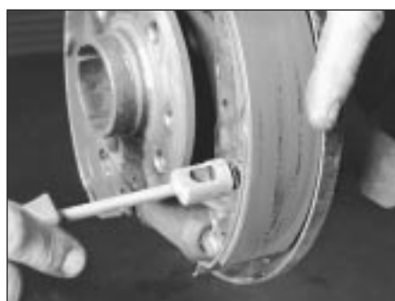
6.6b . . . and the rear shoe hold-down spring
