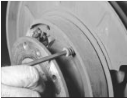
12.7c Remove the shoe hold-down springs
