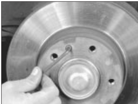
5.6a Remove the disc retaining screw ...
