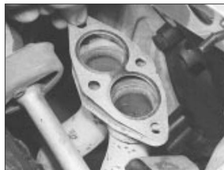
6.7c Removing the exhaust manifold-to-downpipe gasket (M40 engine)
