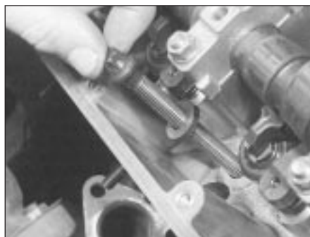
12.29 Inserting a cylinder head bolt (M40 engine)
