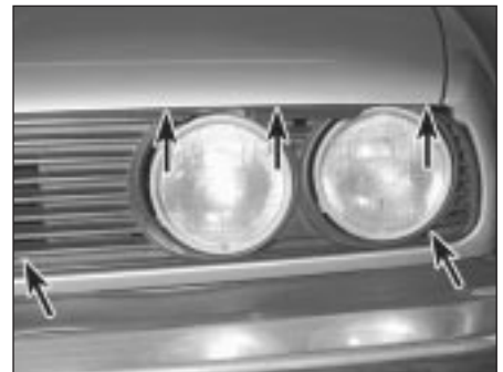
9.2b Side grille screw locations (arrowed)
