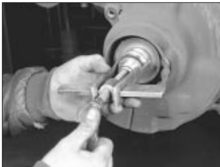
8.8b If the inner race of the bearing sticks to the stub axle, use a puller to get it off
