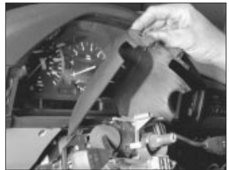
19.5b Rotate the upper shroud up and off the steering column
