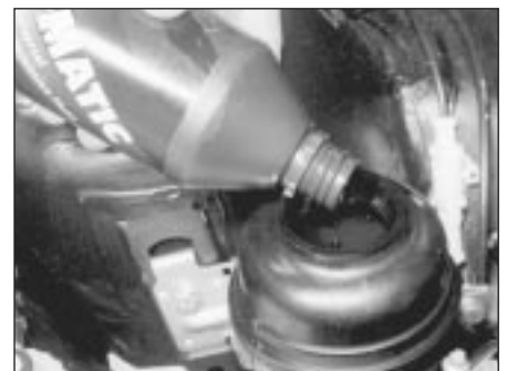
7.6 Adding fluid to the power steering reservoir
