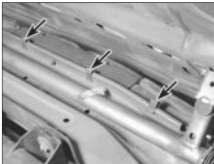
9.1 Open the bonnet and remove the grille retaining clips (arrowed)
