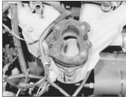
11.10 Carburettor insulating flange on the intake manifold can be removed if necessary
