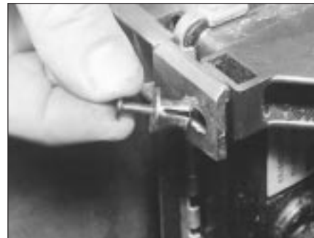
4.5 Plastic fastener retaining the radiator shroud on some engines
