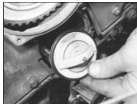
3.20b Removing the thermostat (M40 engine)
