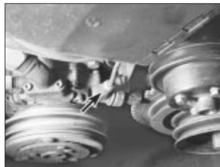
12.10 The pulse sensor itself (arrowed) is located on the timing belt cover, to one side of the pulley (later models)
