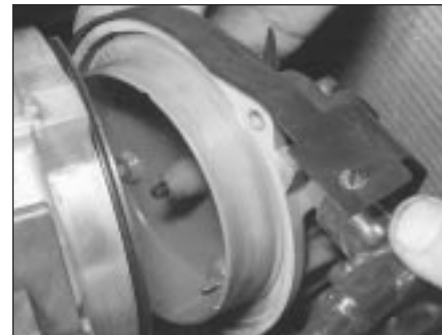
9.6a Unbolt the distributor cap (M40 engine) . . .
