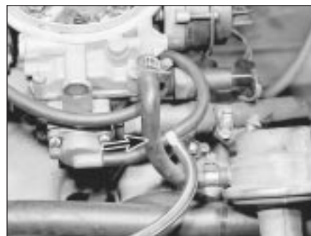
11.8 Disconnect the fuel supply hose (arrowed)
