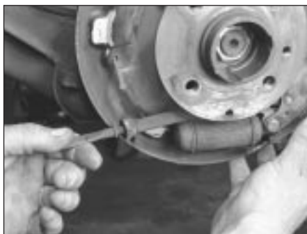
6.8 Remove the automatic adjuster assembly
