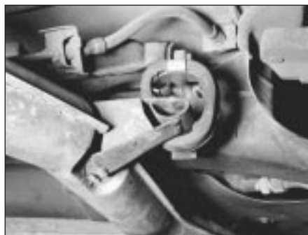
22.1 A typical exhaust system rubber mounting
