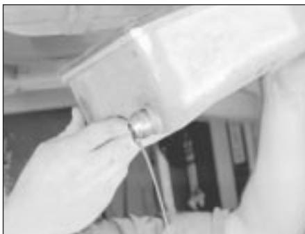
28.7 Lower the sump from the transmission
