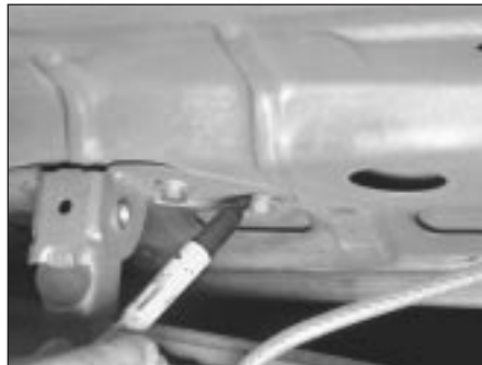
10.1 Use paint or a marking pen to mark on the hinge plate around the bolt heads - mark around the entire hinge plate, if desired, before adjusting the bonnet
