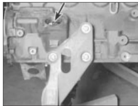
14.4 If necessary on the M20 engine, remove the plug and oil pump driveshaft from the engine. Inspect the driveshaft gear, as well as this intermediate shaft gear in the engine block (arrowed)
