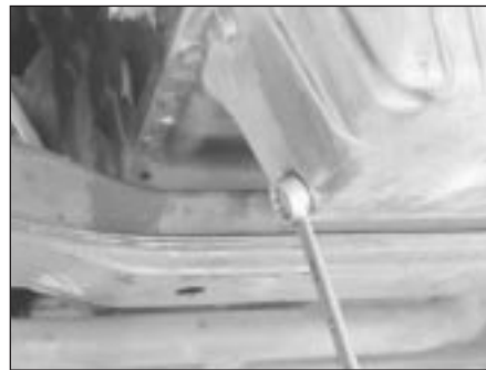
6.7 Using a ring spanner to remove the oil drain plug
