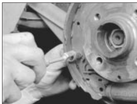
6.6a Remove the front shoe hold-down spring . . .
