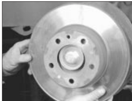
5.6b ... and remove the disc from the hub
