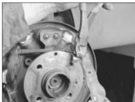
6.9 To disconnect the handbrake cable from the handbrake lever, pull on the plug at the end of the cable, and detach the cable from the bracket on the upper end of the lever (diagonal cutting pliers are being used here because they grip the cable well, but care must be taken not to nick the cable)
