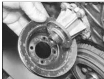
5.29 Removing the water pump pulley (M40 engine)
