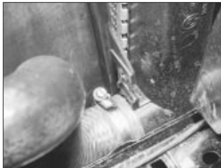
4.3b Bottom hose connection to the radiator
