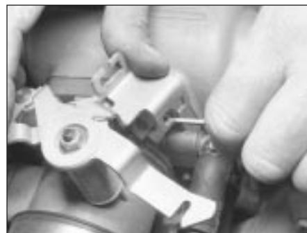
9.10a Rotate the throttle valve and remove the cable end from the slotted portion of the valve
