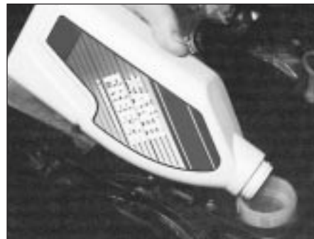
4.9d Adding antifreeze mixture
