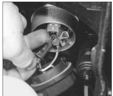
12.11 Removing the headlight bulb (do not touch the surface of the bulb with your fingers)
