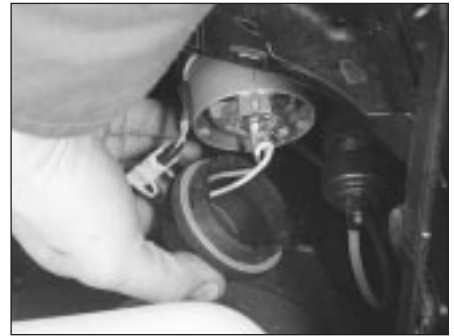
12.9 Twist and release the headlight inner cover
