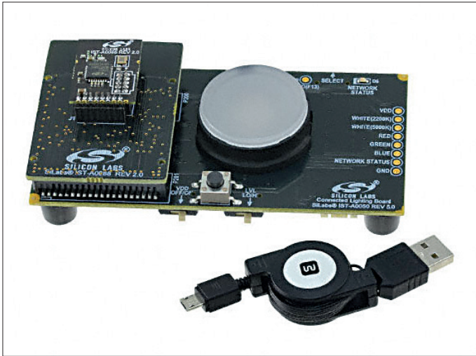
Figure 4. The connected lighting node reference design RD-0085-0401 from Silicon Labs combines a user-programmable EFR32-Mighty-Gecko-based radio module with a sophisticated LED.
