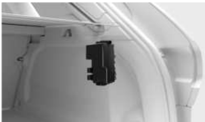
Fuse box location
