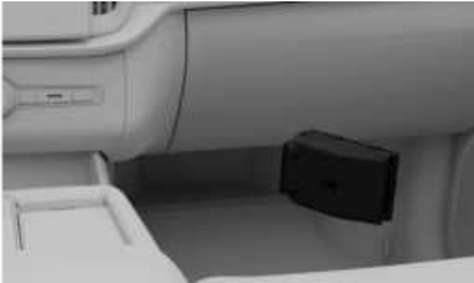
Fuse box location
