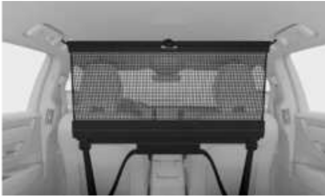
Installing behind second-row seats
