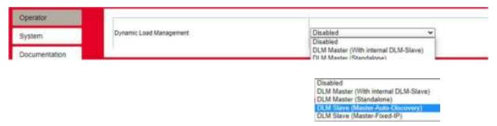
Like the Master Controller more settings will appear underneath, but not as many options. The only setting needed to change here is DLM Network ID, which should be set to the same as the Master, we recommend "1".
