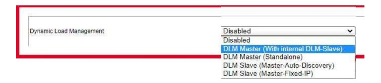
**DLM Master (with internal DLM-Slave)** - This option is for when you have more than one charge point connected on a site. This is only to be selected for the Master side of the charger.
