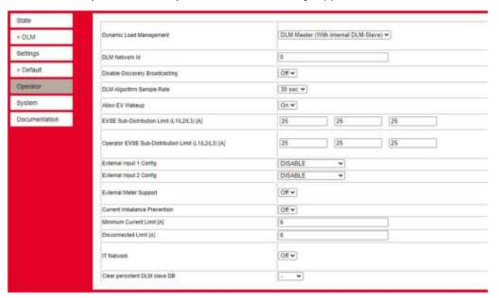
**DLM Network ID** - should be changed to a number for the rest of the chargers to find it. We recommend using "1".
