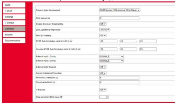
**DLM Network ID** - should be changed to a number for the rest of the chargers to find it. We recommend using "1".
