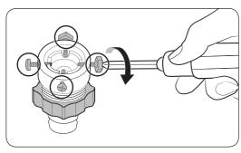
**2.** Use a Phillips screwdriver to loosen four screws on the adaptor.
