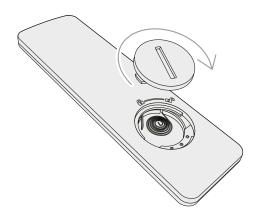
1) Turn the battery cover toward an open-lock image and remove it.
