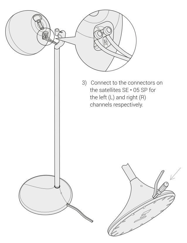
4) Adjust the cord length so that it is not seen from under the satellite. To pull the cord down and loose the locating fixture, use a screwdriver in the manner the picture shows.
