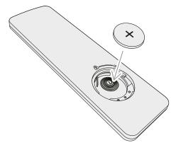
2) Place a R2025 battery, considering the polarity (+ is upper).
