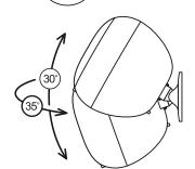
7) If necessary, you can adjust the slope level and angular rotation toward the listener. For this purpose, move the satellite up/down or rotate it right/left.
