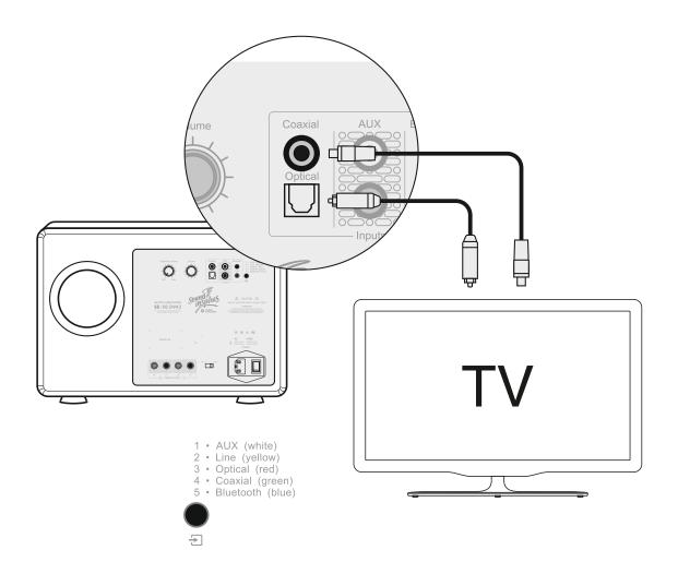
Use a remote control or a back-panel switcher to select a necessary source to play from. The front panel LED should turn a relevant colour: **red** - for Optical, **green** - for Coaxical.
