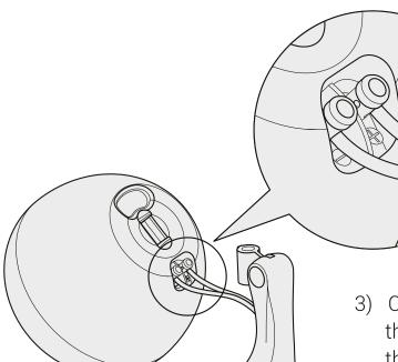
3) Connect to the connectors on the satellites SE • 05 SP for the left (L) and right (R) channels respectively.
