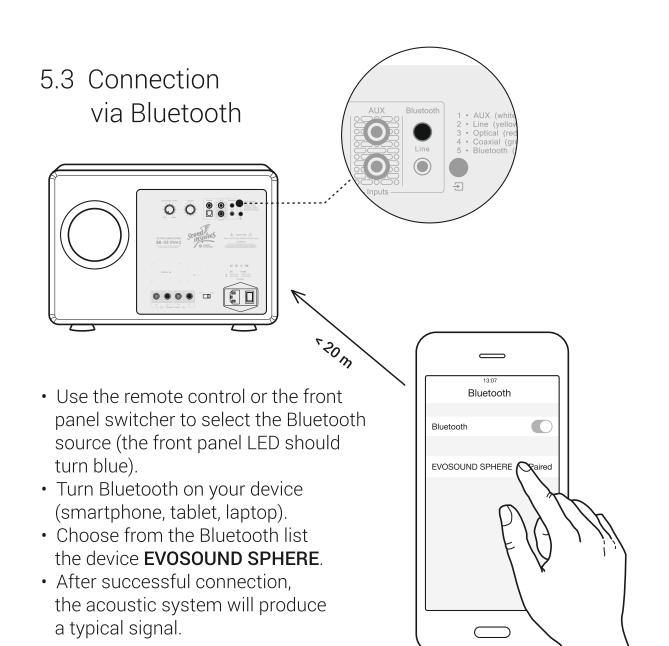
If there is no EVOSOUND SPHERE in the list of the devices, press and slide down the Bluetooth button on the back panel of the subwoofer and try again.
