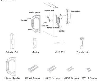
**NOTE:**The lock is suitable for doors up to 2.2 inches in thickness. If you have a new door without a pre-drilled hole, please use the template (included in the package) to drill the new hole. You may also require an electric drill, a pencil, and a hammer.
