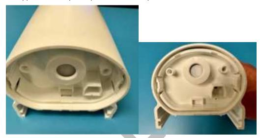
Step 3.1.3 completes the connection of the radio and sensor module with the power module. The subsequent steps can be performed within Hazardous Zones, if needed.
