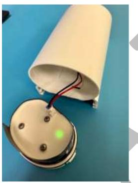
3.1.2. Align the radio and sensor module and the power module and begin sliding the two together. The radio and sensor module will fit inside of the power module.
