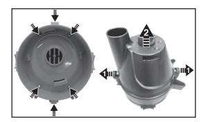
4) Unfasten 6 screws and detach the cover to expose the PCBA, motor assembly, and battery pack.
