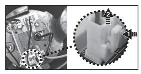
6) Unfasten the 3 screws to remove the battery compartment cover and then remove the battery pack. NOTE: Wrap the connector immediately with insulating tape in order to avoid short circuit caused by contact of both wire terminals.
