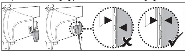
3. Connect the external adaptor to the power source. Once the pool vacuum begins charging, the indicator light on the external adaptor will turn red. Normally, it takes about 5-6 hours to reach a full charge. The indicator light will turn green when the pool vacuum is almost fully charged.
