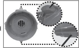
3) Use the screwdriver to unscrew the 6 screws located on the top plate and then detach it from the rear body to expose the rear body's cover.
