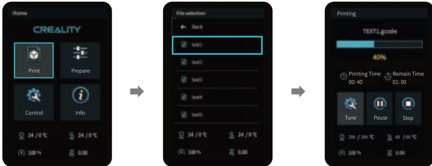
Select the Gcode file you want to print and copy it into the root directory of the SD card. Place the SD card in the printer and from the Print/ file selection menu select the file and Tap The file will start to print.
