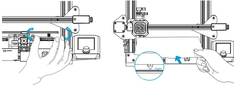
The levelling points are about 30mm in from each corner. There is no need to measure exactly.
