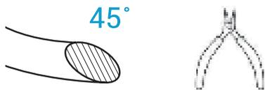
To allow the filament to feed smoothly cut an angle on the end of the filament (as shown above) to help it enter the extruder.
