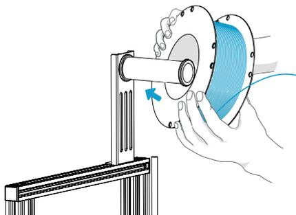
1. The Nozzle must be hot to add, remove or change filament so preheat the nozzle before starting. Hang the filament spool on the holder so it feeds over the top of the spool towards the extruder..
