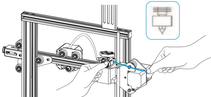
2. Press the lever on the extruder to separate the toothed gear and the idler. Insert the filament into the hole in the lever, between the gear and idler and into the hole on the other side. Keeping the lever pressed push the filament through the Bowden tube and into the hot end and nozzle. As long as the Nozzle is hot enough the filament should start to come out of the nozzle and the filament is successfully loaded.
