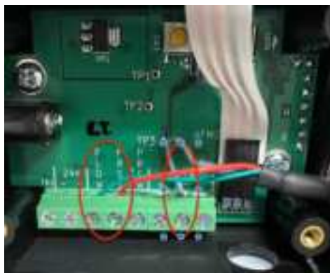
Figure 5 Insertion of wiring into CDI flow meter with Flow and Pressure outputs
