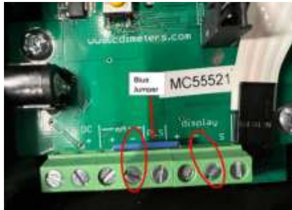
Figure 4 Insertion of wiring into CDI 5200 flow meter with Flow output only
