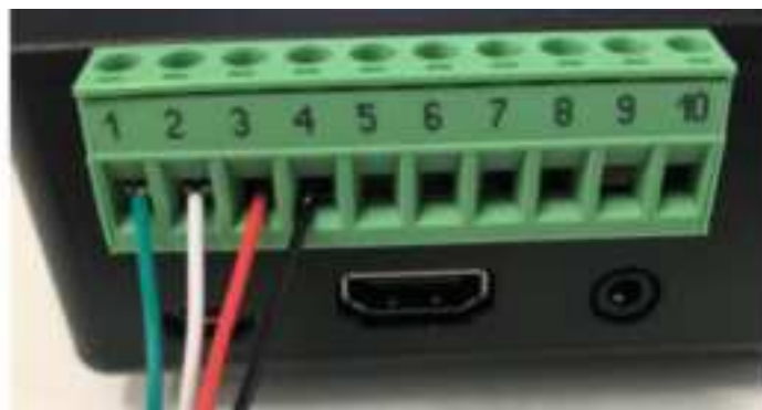
Figure 7 Wiring into the Element-C for flow and pressure measurements
