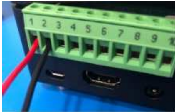
Figure 6 Wiring into the Element-C for flow measurements only
