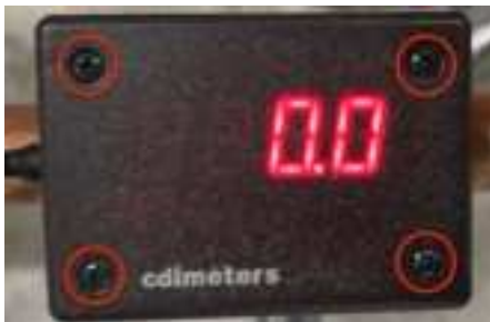
Figure 1 Unscrew the four screws (circled) on the cover of the CDI meter
