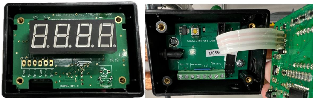
Figure 3a (left): Display board. Figure 3b (right): Output board located underneath the display board
