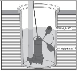
4. Test operation by filling the basin above the Float Switch Operation ON Height to make the pump start pumping out. When the water reaches below the Float Switch Operation OFF Height, ensure it stops pumping.
