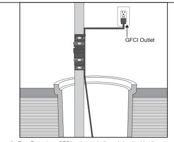
Plug Pump in to GFCI outlet on dedicated circuit with 15 amp breaker
