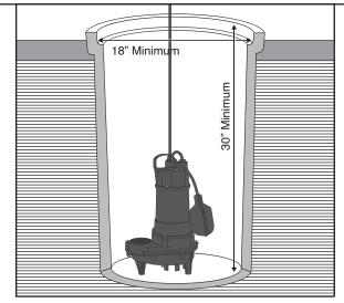
1. Ensure basin is clear of all debris and place pump on hard level surface (not dirt or gravel). 30" x 18" minimum basin requirement.
