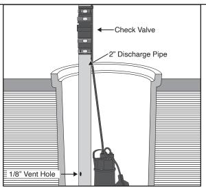
Measure, cut and install discharge fittings, check valve, and piping.
