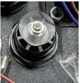
9. Attach the sensor module to the spinner body, ensuring it locks into place in the correct orientation.
