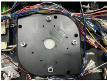
b. Detach the trackball, noting its orientation for reinstallation.
