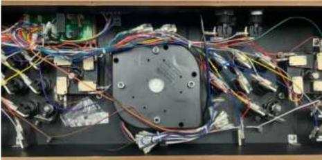
12. Retrieve the PCB and spinner cables provided in the kit. Plug the two spinner cables(A) into the designated ports on the PCB.
