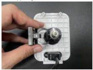
2. Unscrew and remove the nut.
