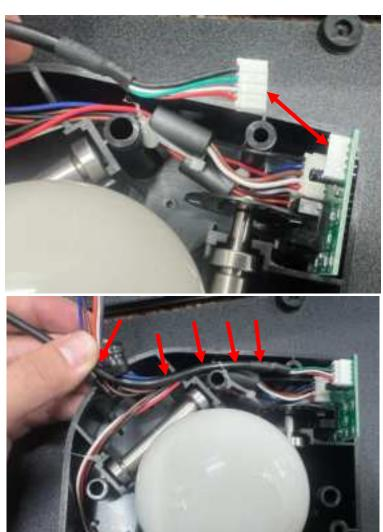
g. Reassemble the trackball, ensuring screws and nuts are tight and the orientation is correct.
