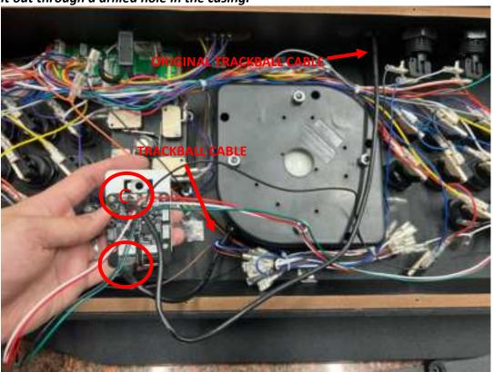
14. Tidy up the internal wiring, ensuring nothing interferes with components. And place the PCB securely inside the Tankstick, avoiding obstructive areas.
