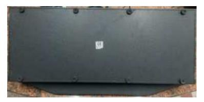
2. Use a flat-head screwdriver to remove the 8 rubber caps (if present) covering the screws.
