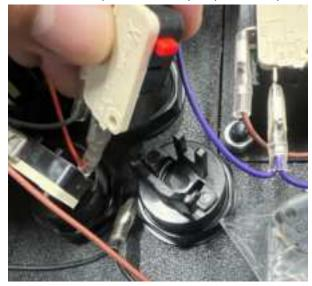
7. Unscrew and remove the selected pushbuttons.
