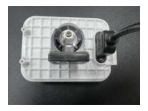
1. Remove the sensor module by pulling it outward to the side.
