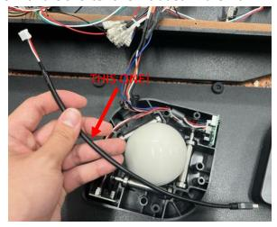
f. Reconnect the cable to the PCB and secure it in the cable clamp. Ensure no cables are pinched.
