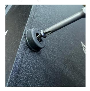
4. Carefully pry the backplate open using a flat-head screwdriver. Set the backplate aside.
