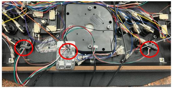
13. For Tankstick with trackball unit, connect the trackball USB cable to any USB-A port on the PCB. And plug the original trackball cable 4pin connector into the PCB Port C as indicated below. For Tankstick Duel/Solo, use the longer USB cable from the kit, routing it out through a drilled hole in the casing.
