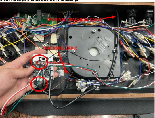
14. Tidy up the internal wiring, ensuring nothing interferes with components. And place the PCB securely inside the Tankstick, avoiding obstructive areas.
