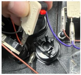
7. Unscrew and remove the selected pushbuttons.
