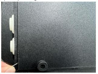
5. Choose two spots for the spinners. You can either drill two 28mm holes, or replace two existing pushbuttons with spinners (as demonstrated in this guide).
