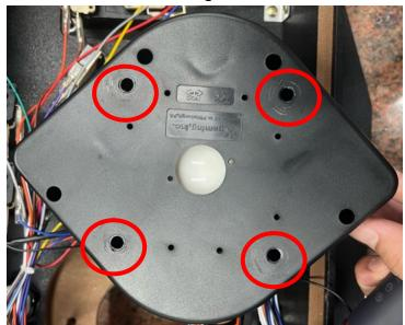
d. Carefully separate the housing, remove the cable clamp, and unplug the USB cable from the PCB.
