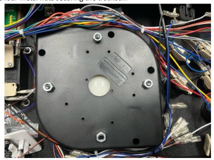
b. Detach the trackball, noting its orientation for reinstallation.
