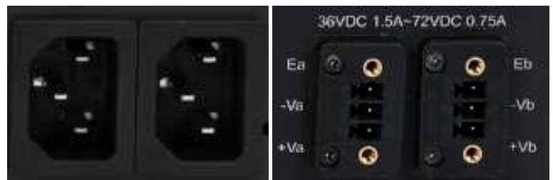
Figure: Dual power supply connectors for OM2200
