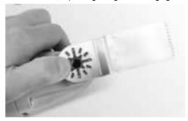
3. Align the perforated end of the scraper with the installation hole. Place a gasket at the point where the scraper aligns with the hole. Secure the assembly by tightening the screws with a hex key.
