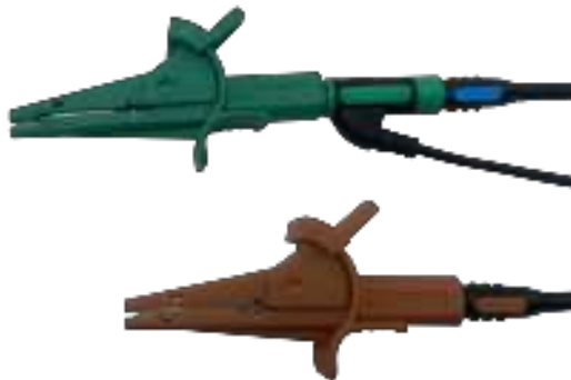
Fig 4. Crocodile clips in 2 wire testing configuration
