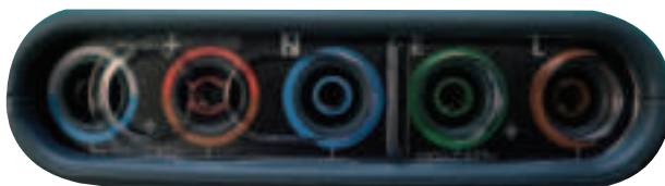
Fig.2 Interlock in position for RCD & Loop testing
