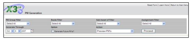
PM Work Orders are manually generated with the menu item called 'Generate PM Work Orders' or the 'Manually Generate' link on the individual PM schedules. When using 'Generate PM Work Orders' (shown above) indicate the date through which the PM's should be generated. It is optional to utilize any of the filters. To preview the PM's that are due to be generated through the date indicated, click 'Proceed.' The list of PM's to be generated will appear on screen.
