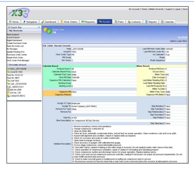
The Calendar Freq. Type determines when the Next PM work order is due to generate. It can either be "Static" (the default setting) or "Shadow". Static PM's are based on the date of the last PM work order that was generated from the schedule. The next PM will generate based on the appropriate frequency listed, counting from the date of the last work order.
